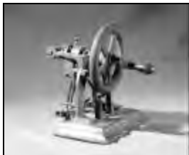
Sewing machine patented in 1846 by Elias Howe Jr.
