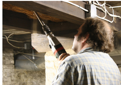
Dan Miles of Oxford Dendrochronology Laboratory taking a core sample at the Hooper-Lee-Nichols House
